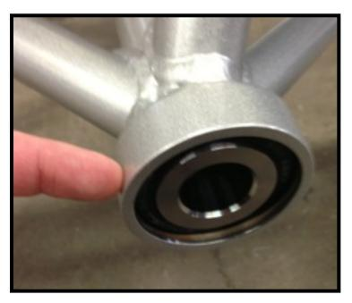
INSTALL GREASE FITTING ON THE BACKSIDE OF THE BEARING CUP TO KEEP ROCKS, DIRT AND ANY FLYING DEBRIS FROM DAMAGING IT
